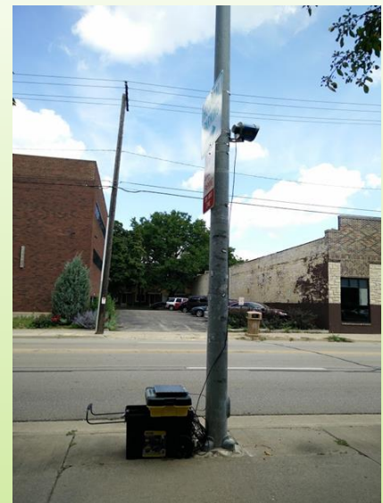
Typical installation of radar-based data collection equipment used to obtain vehicle trajectories
